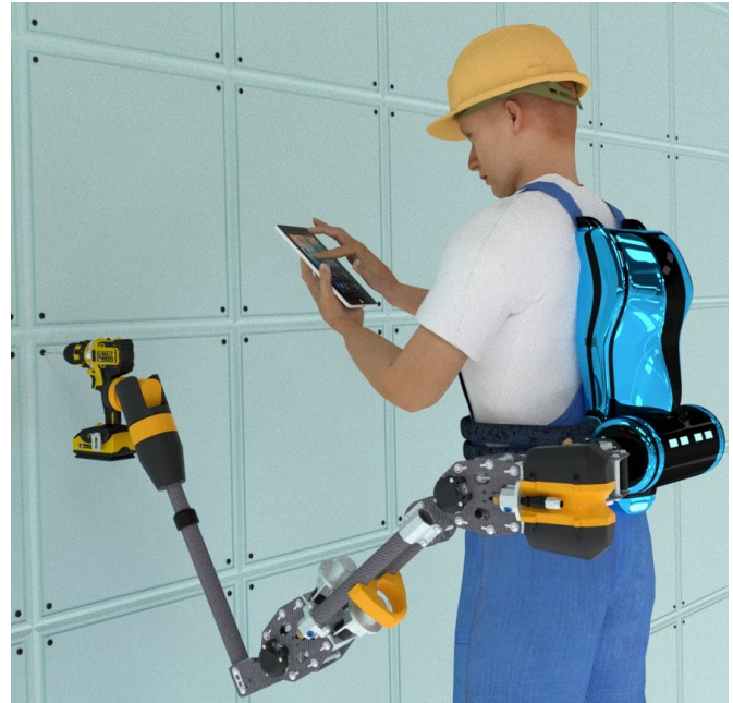
Fig. 1. Worker wearing a SRL for automatic machining operation
