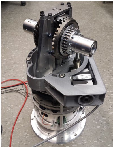
Fig. 16. Assembled manipulator base with the load cell mounted on the supporting frame.
