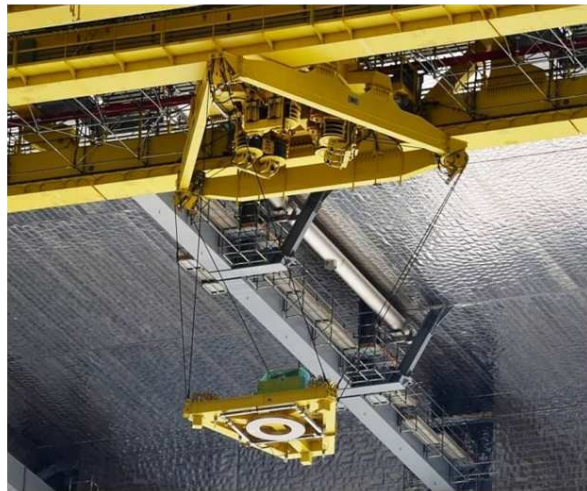
FIGURE 1.1 – Le NIST Robocrane.(Photo provenant du site web : https://www.nist.gov/nist-time-capsule/fixe-life-nist-help/helping-clean-disaster-inside-chernobyl-mega-tomb , consulté le 08/04/2019, Auteur :Chernobyl Nuclear Power Plant)
