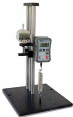
Force One™ FDX mounted on Wagner STK100 Spring Tester
