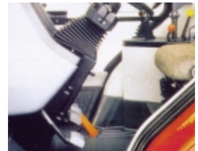
Picture 2.6: iglide® G300 plain bearings have proven themselves in control levers and pedals of farm tractors and construction vehicles
