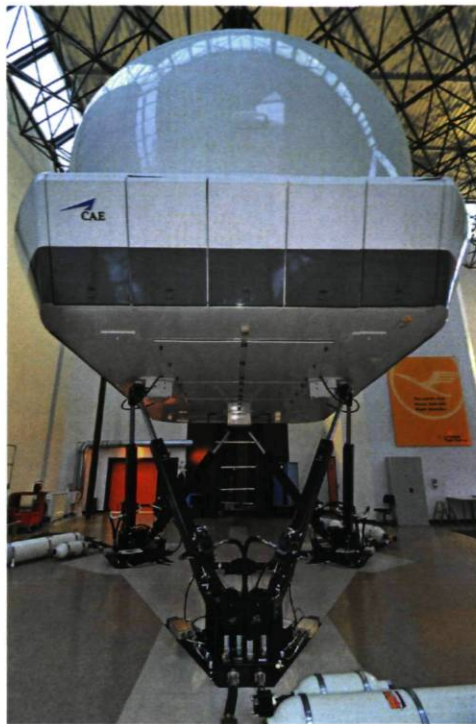
Figure 1.7: A CAE flight simulator based on the concept of Gough-Stewart platform “Courtesy of CAE Electronics”.
