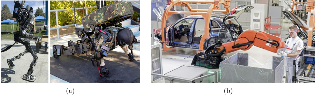
Figure 1.2 – Support of humans in heavy works: (a) A human is equipped with an exoskeleton developed by Sarcos Inc. [SARCOS]; (b) Human-robot cooperation in Audi’s production.
