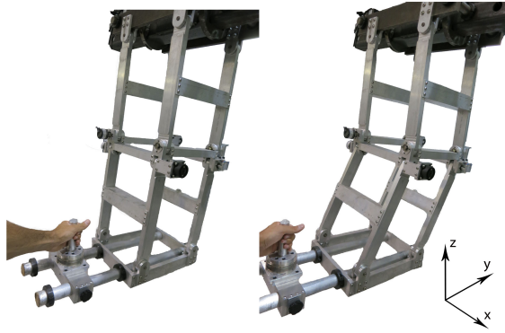
FIGURE 4.21 – LIP (mini) component of the macro-mini robotic manipulator attached to a 3-dof gantry structure (macro, not shown here). This architecture allows the x and y horizontal motions.
