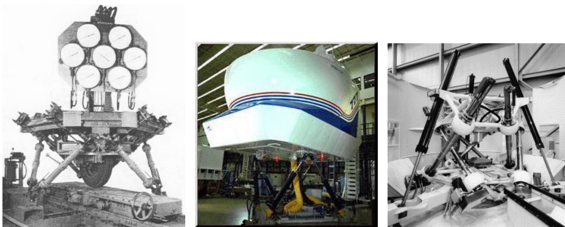
(a) Gough's tire testing machine. (b) Flight simulator (CAE Electronics Ltd, Canada). (c) Parallel kinematic machine (Giddings & Lewis).
