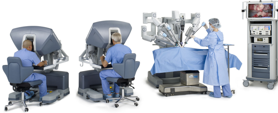
Figure 0.7 – The well-known master-slave da Vinci® Si Surgical System (laparoscopic surgery).
