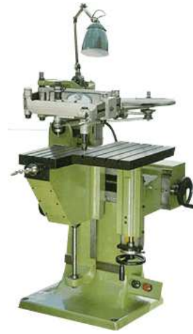
(b) A market-available three-DoF pantograph
