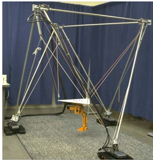
Figure 1.2 – The mobile 2 m octahedral gantry frame RoboCrane mounted to three skid-steer trucks.
