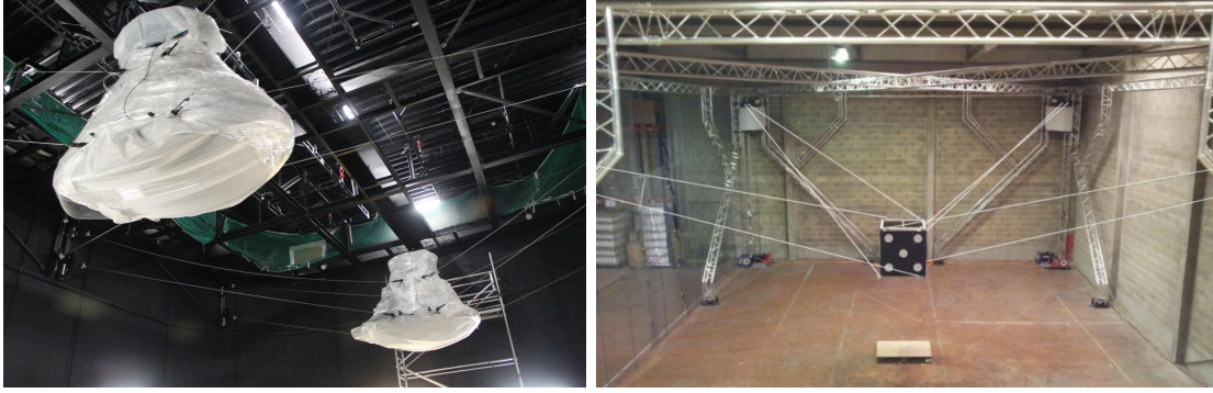
Figure 1.6 – Cable robots in the German Pavilion at the World Exhibition EXPO 2015 in Milan. Figure 1.7 – CoGiRo: A large-dimension cable-driven parallel robot.
