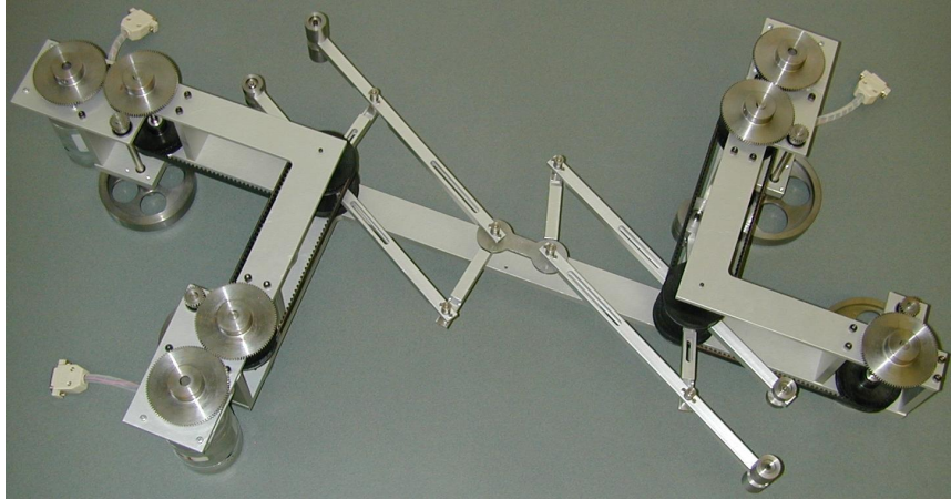
Figure 1.5: Prototype of a reactionless planar 3-DOF parallel mechanism (from Foucault and Gosselin, 2002).
