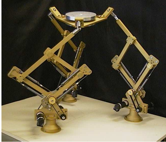
Figure 1.4: Statically balanced parallel manipulator (from Gosselin et al., 1999).
